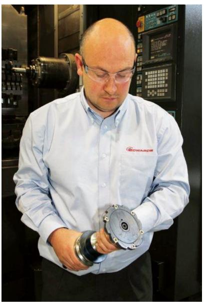
Three side-milling cutter bodies of different diameters were supplied to accept 10mm-wide, ground, coated-carbide indexable inserts for either roughing or finishing, the latter inserts being developed especially by AVANTEC for the application. The smaller cutter accommodates five inserts on each side, while the other two bodies have six inserts per face, all secured in deep pockets that expose only the edge of the inserts.
