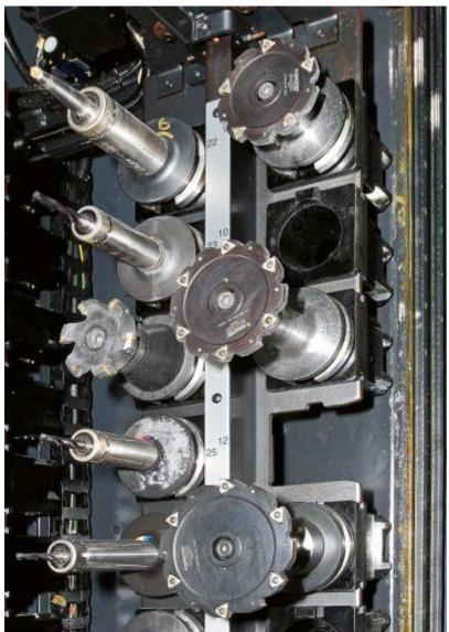
The new process using the AVANTEC cutters consumes just 6% of the original cycle times. As chamber milling (roughing plus finishing) used to account for around two-thirds of the total program run time on a casting, the 94% reduction translates into a 60% reduction in the overall cycle.
