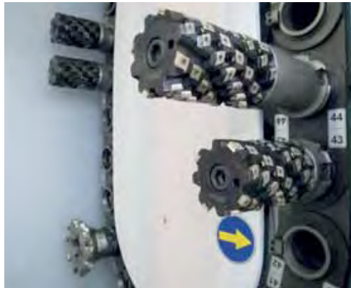
Detail of the so called hedgehog milling tools used to machine the steel beams
