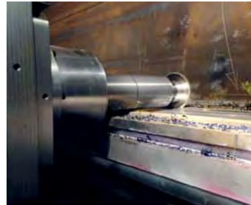
Machining of the channel of the bearing seat with a Avantec disc miller
