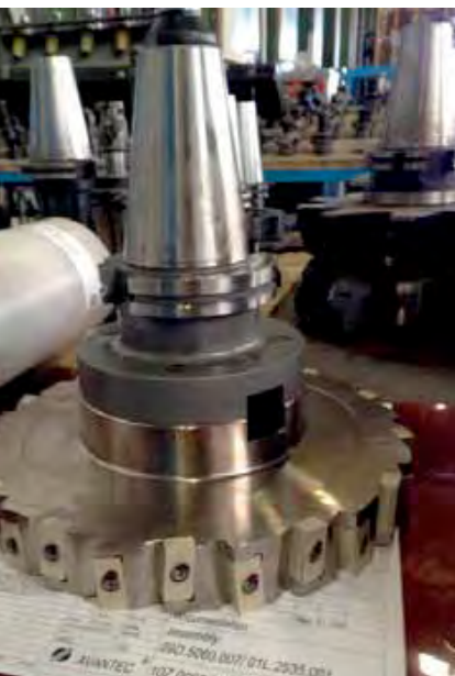
right side: shell end cutter for the rough machining of the steel beam made at Industrie Meccaniche Cimolai
